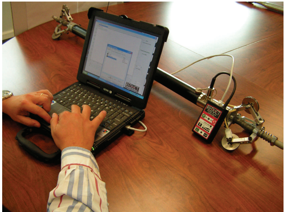
Downloading survey data from the PipeTrack unit after completion of a pipeline survey.
